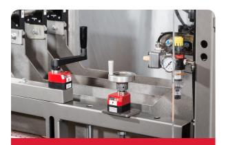
Changeovers are repeatable and toolless with pointers and digital scales
