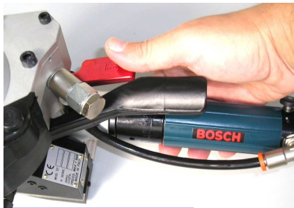
PHASE 2; SEALING AND CUTTING THE STRAP
