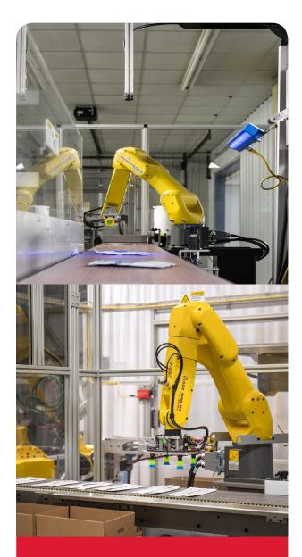
Advances in vision sensor technology and end-of-arm tooling has evolved into more nimbler product handling for case packing.
