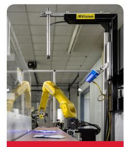
Advances in vision sensor technology has led to the development of a variety of end-of-arm tooling that has evolved into more nimbler product handling for case packing.
