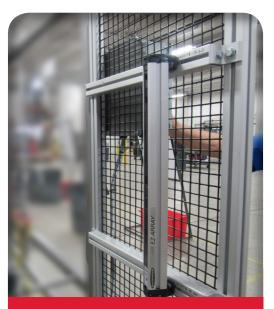
A light curtain senses the height of the incoming case, communicates with the servo and the height of the top taping head is automatically adjusted.
