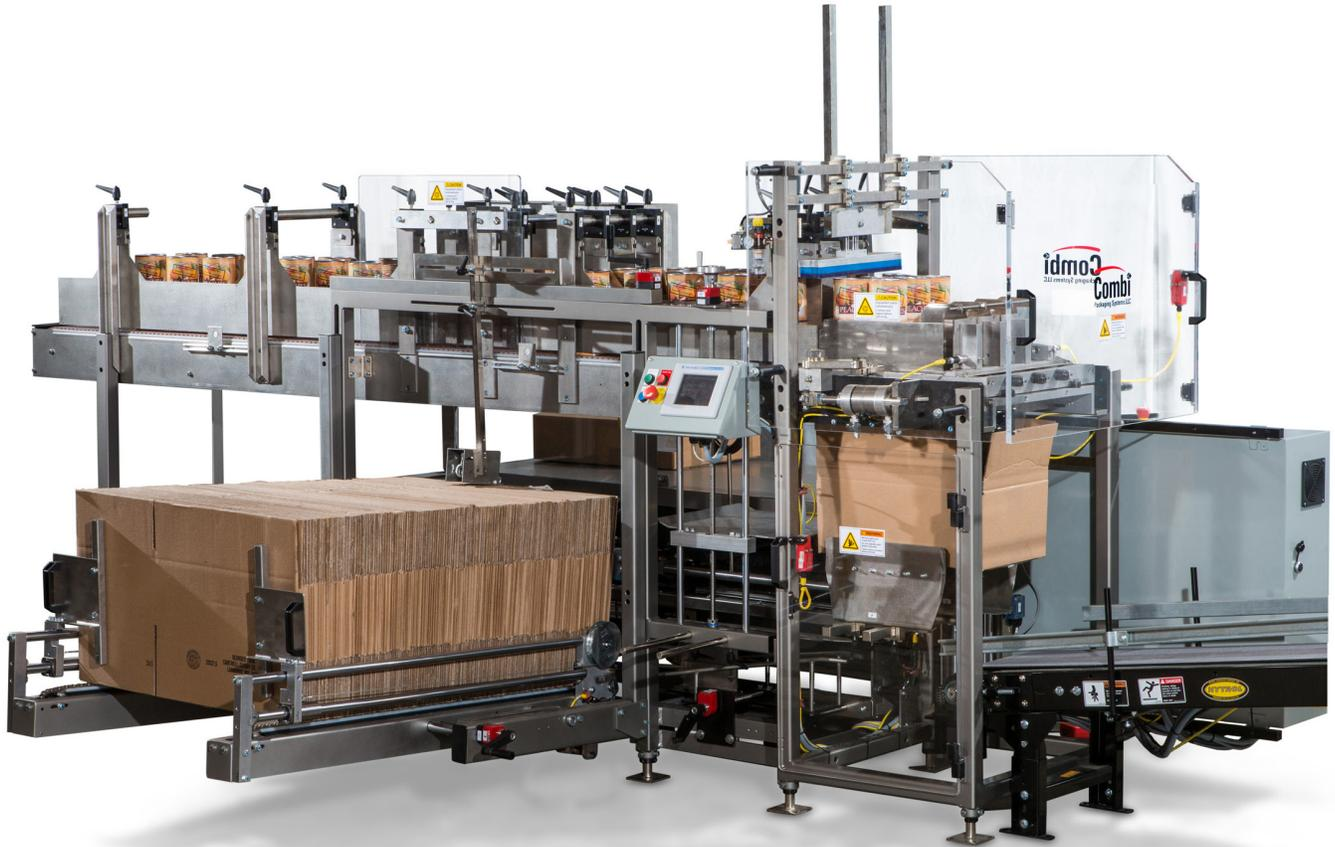
With over 39 years of design and innovation, the Combi DP Drop Packer continues to evolve into one of the industry's most reliable and robust case packing machines. Built into the strongest frame and resulting in one of the smallest footprints in the industry, is a convenient walk-in case magazine and case erector. Setup and changeovers are simple and fast with our modular, slide-in packing heads and quick-clamp product lane guides.
